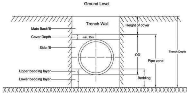
Usually, the minimum bedding is according to EN1610  $a = 100\text{mm}$ , in case of bedrock or compacted
