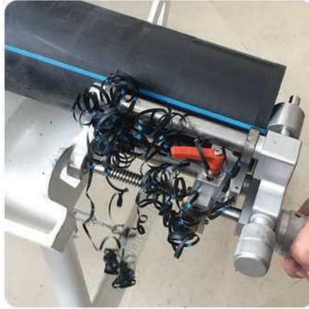
2- Scrape at last 0.2 mm of outside pipe surface to remove oxidation and other contaminants.
