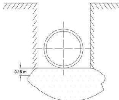
The crucial factor to attain a good load capacity of pipes and fittings underground is a correct construction of the area around the pipe. The correct design of the pipe zone is determining the load capacity of PE pipes and fittings.
