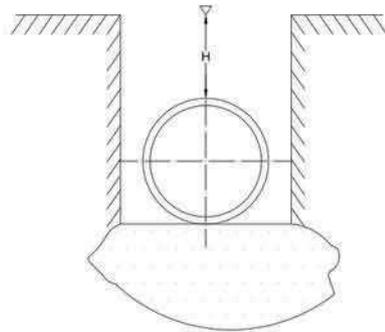
The base of the trench has to enable the pipeline to bear on smoothly. In case of bedrock the trench has to be excavated deeper and filled to the desired depth with appropriate material which grain size does not damage the pipe.
